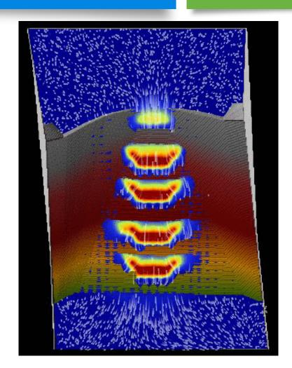
Comparison of Fish Ramp Simulation to 10% sloped ramp with channel through center
