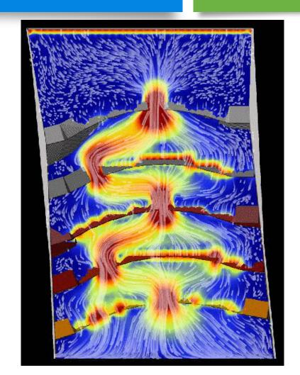
Comparison of Fish Ramp Simulation to 10% sloped ramp with channel through center
